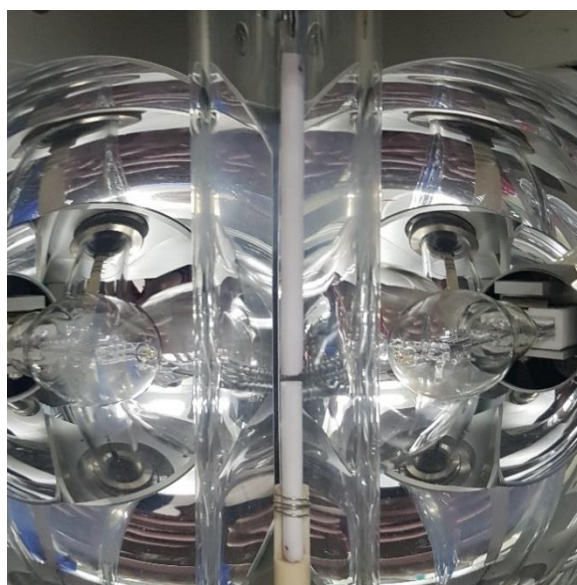
Fig. 1. Growing of \text{Tb}_2\text{Ti}_2\text{O}_7 single crystal by the optical floating zone technique
